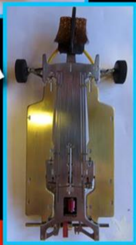
New castricone 2015 F1 chassis. An ope rear end following a trend set by Richard Mack.
